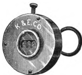
FIG. 37.—Tally Register. This instrument consists of a metal box or case about 2 inches in diameter and \frac{1}{2} inch thick, containing a mechanism including three numbered wheels the edges of which are exposed through a small glass disk set in the center of the front of the case. The wheels are turned step by step by a plunger projecting through the edge of the case in position to be operated by the thumb. The box is carried within the palm of the hand and held by a ring through which the middle finger is passed. It counts from 1 to 999 and costs $2.50. (See Fig. 37.)
