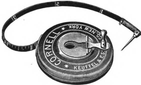
FIG. 5.—Tape for Measuring Girths and Diameters.
